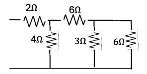
Step 2: combine  $3\Omega$  and  $6\Omega$  resistors [parallel]:  $(1/3 \Omega + 1/6 \Omega)^{-1} = 2 \Omega$
